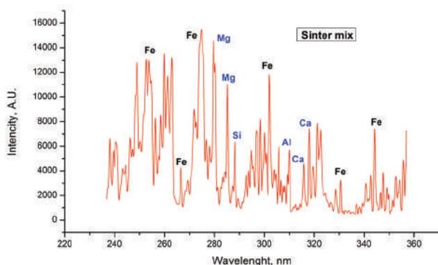
**LIBS analysis process:** a laser beam is focused on the surface of the material directly on the belt with a high frequency, generating a plasma at that point. Then, the plasma quickly cools down and the excited ions return to the low energy state, emitting characteristic optical radiation. Based on the obtained spectra, the concentrations of all the necessary elements and compounds can be calculated simultaneously and directly, obtaining the results in a real-time mode.
